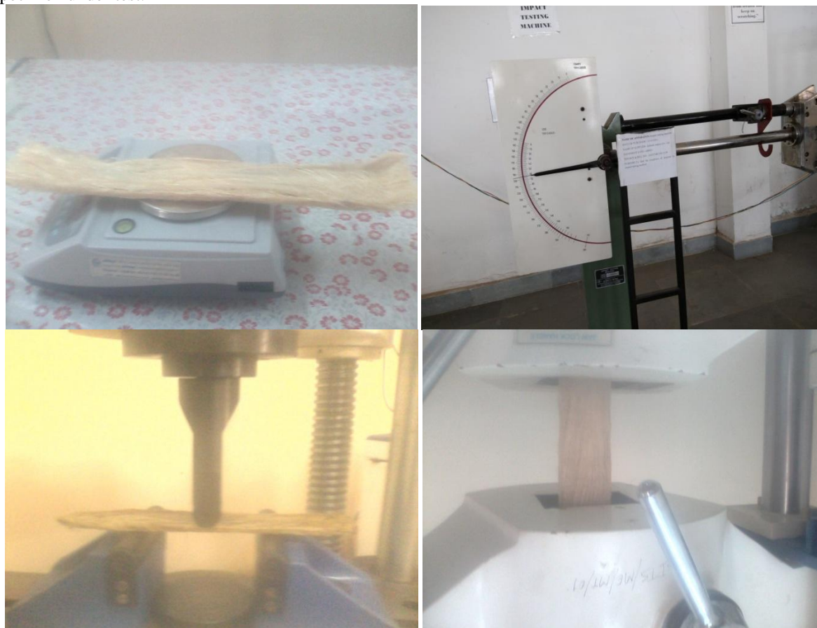
Figure 2.4 Composite Sample weighing & Mechanical Testing
