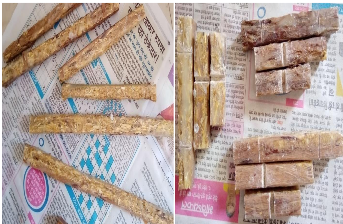
Figure 2.3 Open mould system used for making composites & Sample Preparation
