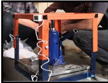
Figure 2. Self-Made compression moulding set-up
