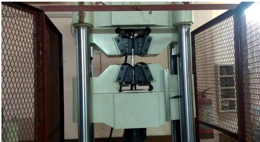
Fig.6. Setup of tensile testing
