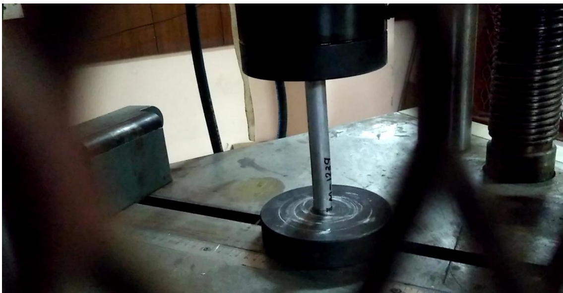
Fig.2. Setup of compressive testing
