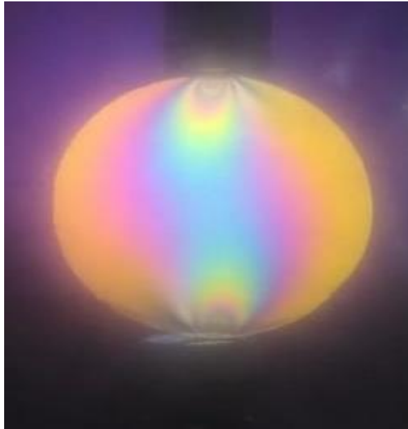
Fig. 3: Fringe formation in Model - 1 under compression observed in polariscope using white light.
