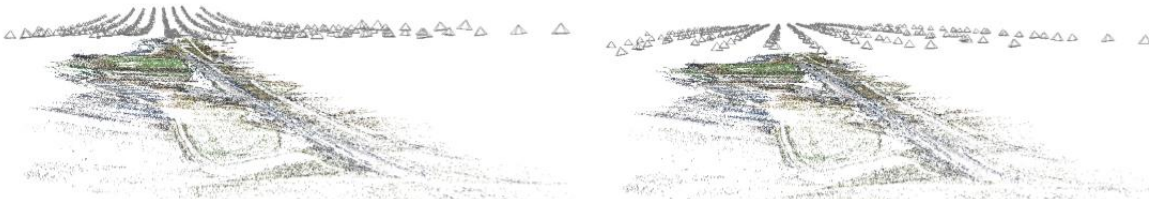
Fig 7: Effect of Bundle Adjustment (Right) source google precise measurements of the sensor position and orientation exactly at the time of exposure or scan.
