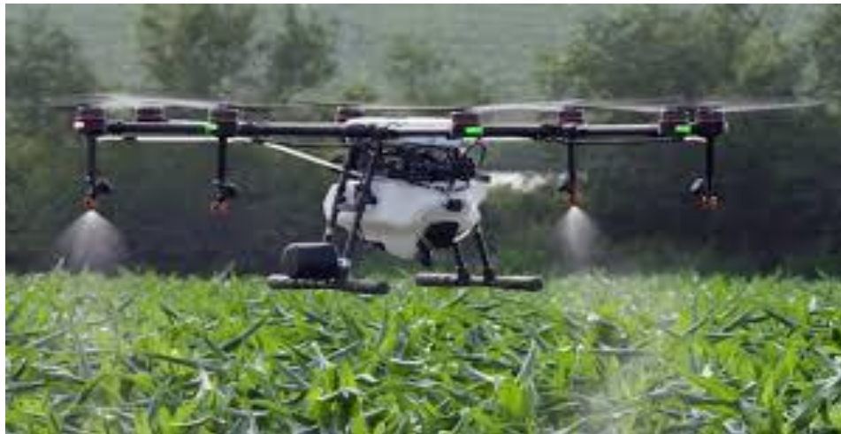
Fig 5.2. 7: Spraying pesticides using quadcopter source google
