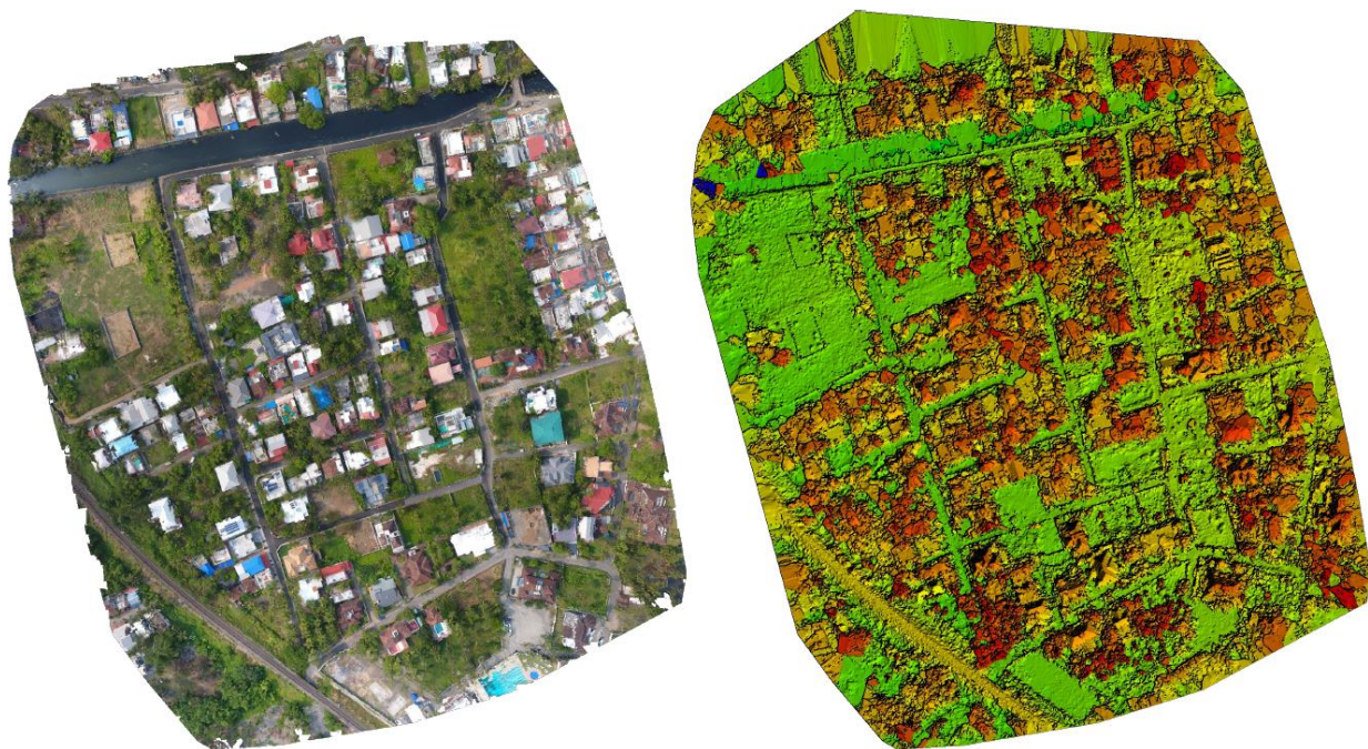
Figure 5.1.3 Orthomosaic and the corresponding sparse Digital Surface Model (DSM) pix4dmapper before densification
